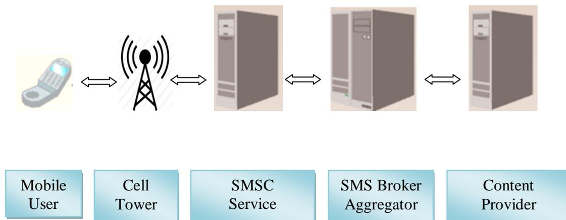
Figure 1: Process of Communication between a Mobile User and a Content Provider
