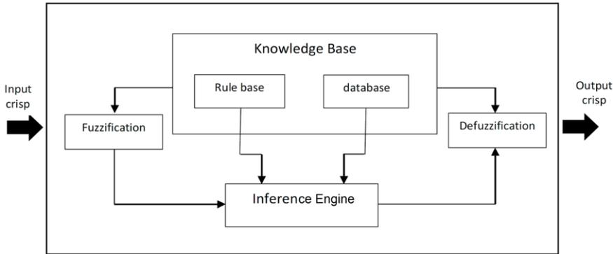
Figure 1: Block Diagram of FIS
